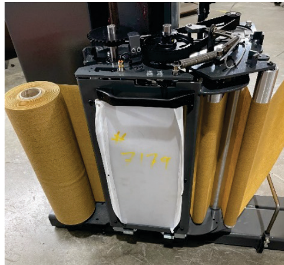
Paper Wrap Material Running on a Phoenix Stretch Wrapper (left); Carriage with Paper Wrap Material (right)
